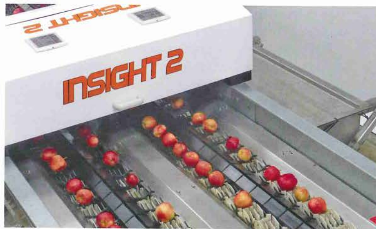
Gala apples entering the pre-sizer's camera module.
