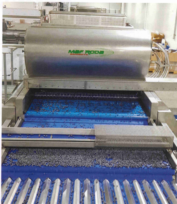
LEFT—MAF Roda's Berryway-Berryscan electronic grader used by Camposol in Peru for sorting and selecting blueberries
